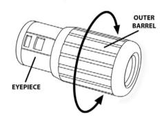
**Note:** The close focus optical system allows you to focus on a subject as close as 10 inches in front of you.
