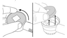
For hands free use, make sure support adapter is attached to the end of the handle so that loupe base will be flush to viewing surface.
