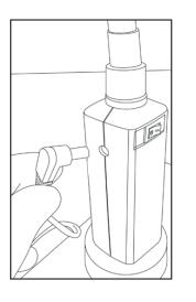
6. Turn on light switch located on the front of the magnifier.
