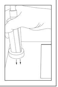
To use with table clamp, place open c-clamp onto a table or hard surface and tighten securely by handle.
