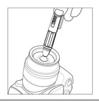
Step 3: Replace cap and twist one half turn to replenish cleaning compound on tip.
