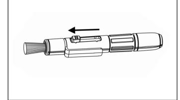
Step 2: Use brush to wipe away loose dirt and debris from lens. Retract brush when done.
