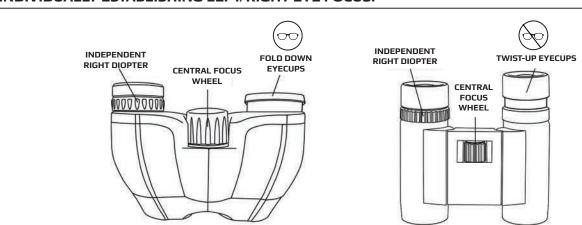
Most binoculars have a center focus wheel and an independent right diopter eyepiece to account for small differences in the strength of each eye. Please follow the steps below to focus properly:
