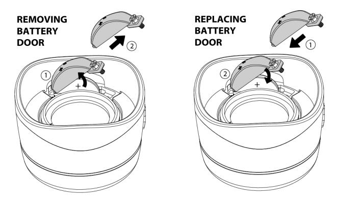
**NOTE:** Battery may be difficult to remove by hand. Needle nose pliers are recommended.
