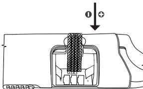
3. Close battery door and tighten with screwdriver.
