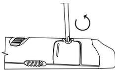
2. Remove used-up batteries and insert 3 new G3 button cells into compartment in the correct polarity.
