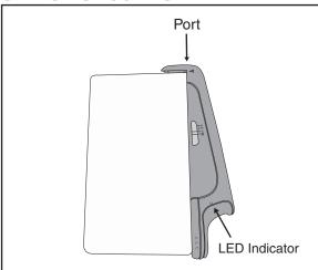
**Before First Use,** battery must be fully charged. Plug the small end of cable into book light's port and the larger end into computer's USB port.
