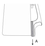
2. Slide clip into position and align the arrow on clip with the arrow on handle (B). It will click into place. Once in place, rest clip on top edge of book (C).
