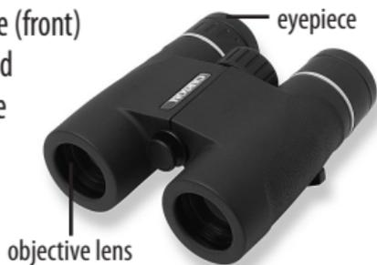
**Porro Prism Systems:** the objective lens is offset from the eyepiece. Light is redirected through the binocular internally. The result is a shorter, stockier shaped binocular. In general, porro prism binoculars offer a wider field of view. Most zoom binoculars use the porro prism system.
